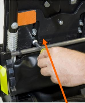
Use the 7/16" nut driver to adjust the trunk supports. There should be 1 to 2" of space between underarm and top of trunk support.
