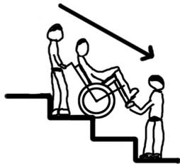
When going down steps, the chair should be tipped back and moved to the edge of the step. The pusher controls the descent of the chair by bending the knees. The second person stands in front of the chair and steadies the chair by holding the front frame (do NOT use the footbed).
