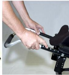
The handle bar is adjustable by changing the position of the snap buttons on the seat back tubes. You can flip the handle bar around for a better handle height by drilling an additional hole to accommodate the snap button.
