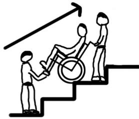
GOING UP STEPS: A **minimum of two people** should be used when taking a wheelchair up steps. Position the chair squarely at the foot of the steps with its back toward the steps. Place one foot up on the first step, and pull the chair up by straightening your legs. The second person stands in front of the chair and assists by holding the front frame of the wheelchair (do NOT use the footbed).
