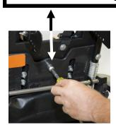
The seat back can be adjusted with a 7/16" nut driver. The seat back has room for 8" of growth. The height of the seat back should not interfere with arm motion or function.
