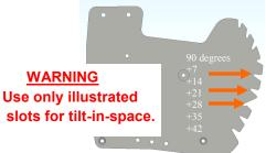
Tilt-in-space will assist the child's muscular trunk control against gravity and aid in pressure relief. If it is too erect, he may slump. If too far back, he may pull forward to become more erect. It is important to position the child as erect as possible to encourage the child to develop the strength and balance needed to improve. As needed, tilt the child back to remove pressure from the buttocks area in order to allow proper circulation of blood
