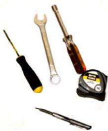
The basic adjustment tools for the ROC Wheelchair are: 7 1/16" nut driver, 5/32 allen wrench, 3/4" wrench for front wheel caster bolt, tape measure, and pen.
