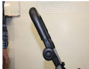
The ROCKIT Wheelchair handle bar is adjustable by pressing the buttons at the base of the handle.
