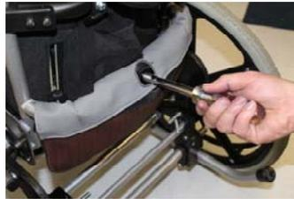
Seat back is adjusted with 7/16" nut driver. **Seat back has 8" of growth.**
